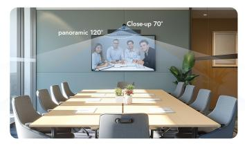
The RB20 features a dual-lens design with a 120° wide-angle 4K lens for panoramic views and a 70° wide-angle 12x optical zoom for detailed close-ups. It also supports dual video with a picture-in-picture display, enhancing the meeting experience.
