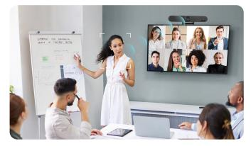
RB20 has a built-in sound localization algorithm. When a participant speaks, the camera will lock onto the speaker based on sound, automatically changing the color of the close-up shot's border to indicate the speaker's position and provide a face-to-face communication experience.
