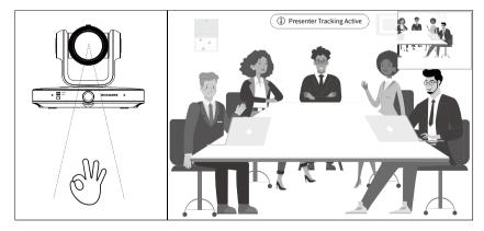
**Step 3** When the tracked person moves, the camera will automatically lock the position and give a close-up image.
