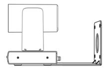
According to diameter and position of the 4 installation holes (As shown below) on the bracket, drill 4 holes on the wall and fix the bracket onto the wall by using 4 screws which should be prepared by you.
