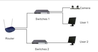
Please refer to the above diagram, user1 and user 2 are in the same router, they are considered as in the same LAN, connect the camera to the same LAN as where the PC is, and refer to below instructions as how to use the application software, then the camera can be found and connected from the online device list.
