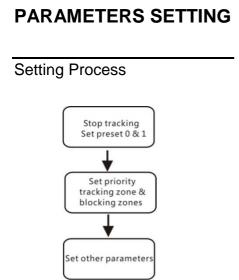
Preset 0 and Preset 1 are set as presets of full view image, or as presets of any zoom or position. When there is no target, camera will return to preset 0 or preset 1. Please refer to Basic Setting.
