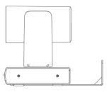
According to diameter and position of the 4 installation holes (As shown below) on the bracket, drill 4 holes on the wall and fix the bracket onto the wall by using 4 screws which should be prepared by you.
