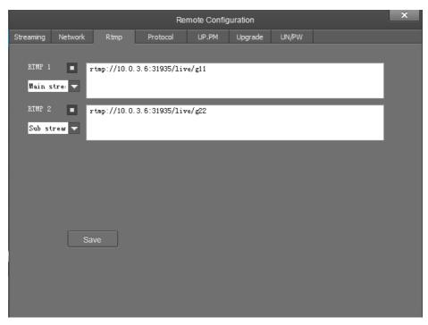
In RTMP1 and RTMP2, main stream, sub stream can be chosen to stream.
