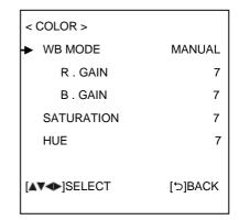
WB MODE: AUTO, ATW (auto tracking), ONE PUSH, INDOOR, OUTDOOR, MANUAL, SODIUM LAMP, FLUO LAMP, COLOR TEMP.
